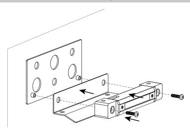
Pass the screws through the holes on the top of the fixture and glare guard into the mount. Tighten both sides firmly with a screwdriver.
