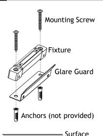
Pass the mounting screws through the holes on top of the fixture and mark both points on the desired mounting location. Drill holes using the marks, then insert the anchors (not provided) into the drilled holes.
