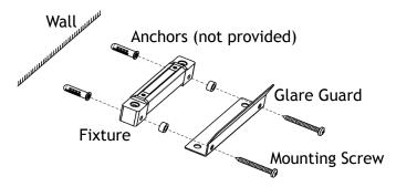
Pass the mounting screws through the holes on the side of the fixture and mark both points on the desired wall surface. Drill holes where you made the marks. Then, insert the wall anchors (not provided) of the proper type into the drilled holes. Pass the mounting screws through the bracket and spacers as shown. Tighten them together by threading the mounting screws into the wall anchors.
